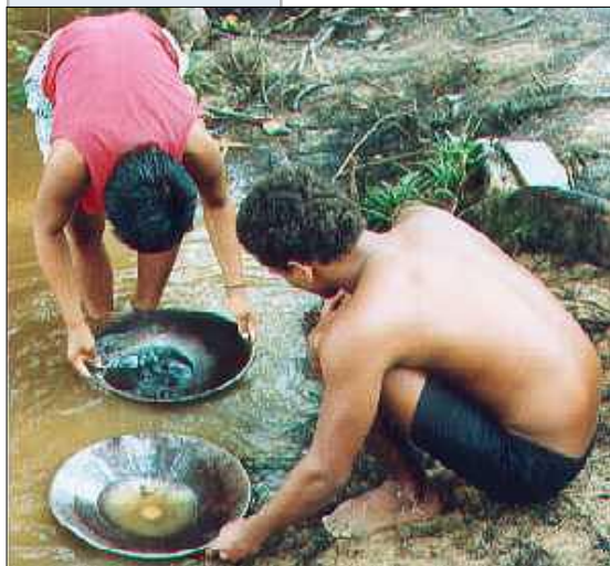
Mercury being mixed in with the gold in the upper pan. Copyright Michael Jorn Mangal
